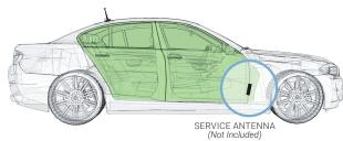
Install **Service Antenna** in the cab, towards the front, where coverage is needed. Ideally, there should be substantial material, like the metal of the roof, between the Donor and Service antennas, to improve isolation.
